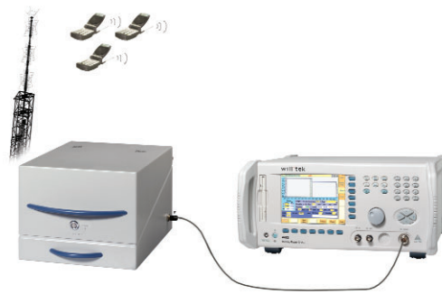
Interference-free testing with RF Shield Box
